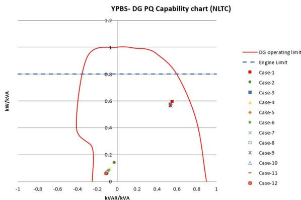
Fig. 4. Generator operating points in the capability chart with fixed shunt reactor applied
