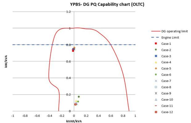
Fig. 5. Generator operating points in the capability chart with variable shunt reactor applied
