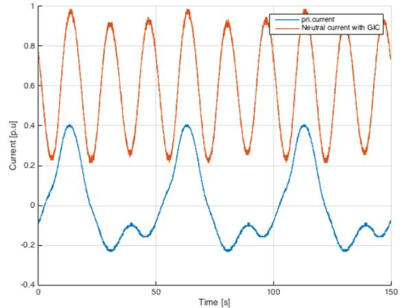
Fig. 4. GIC and no DC flux compensation windings. Primary voltage 230V
