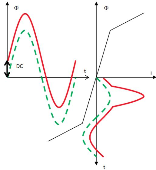
Fig. 1. Mapping from magnetic flux in the transformer core to primary current. Dashed corresponds to without GIC and solid corresponds to with GIC.
