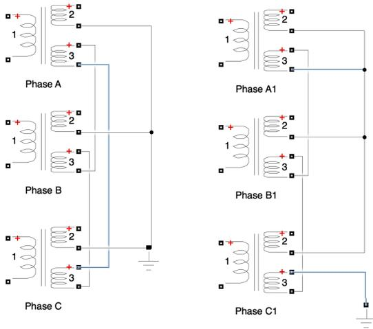
Fig. 2. Reconnection from delta to compensation winding
