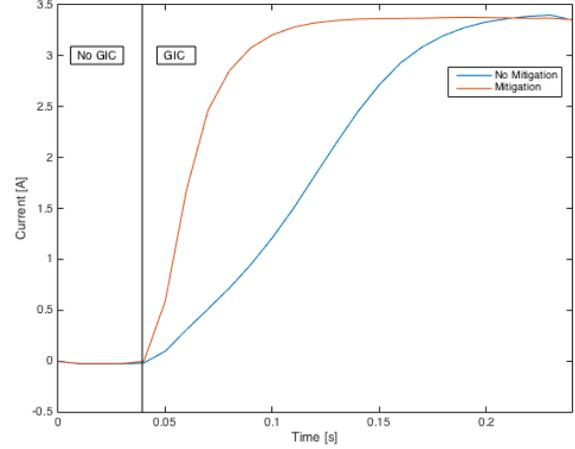
Fig. 6. Step response with and without DC flux mitigation windings. Primary voltage 50V
