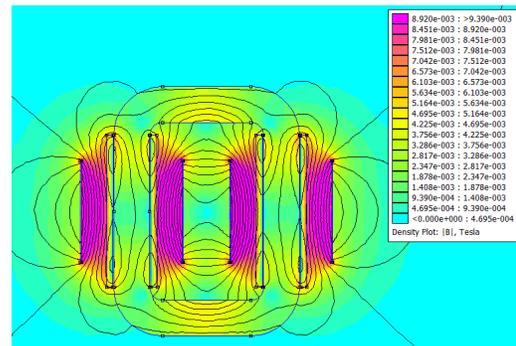
Fig. 3. Short-circuit FEMM simulation
