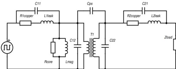
Fig. 1. Equivalent scheme of the pulse transformer
