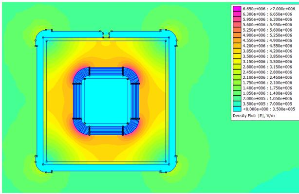
Fig. 7. Electrostatic simulation of transformer cross section in Finite Element Method Magnetics
