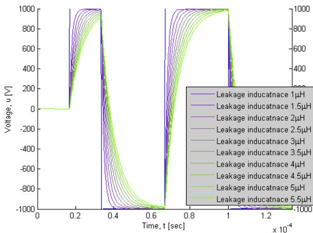
Fig. 4. Influence of leakage inductance on output waveform
