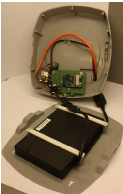
Figure 6 - Internal architecture of the docking station
