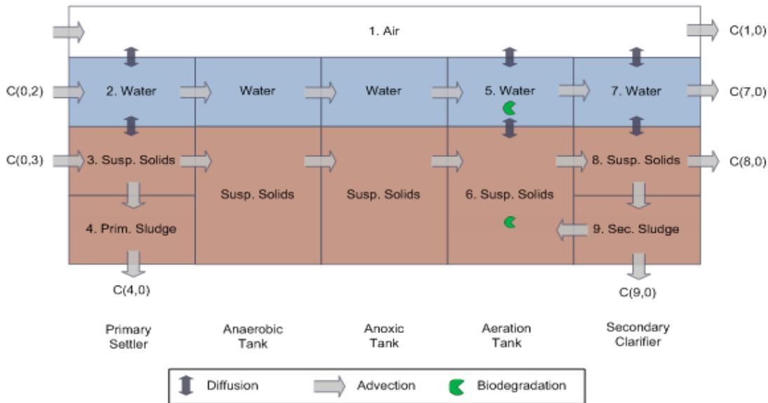
Figure 1. Process scheme of the modified SimpleTreat model.
