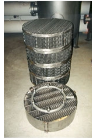
Figure 5.3: The structured package in the humidifier at LTH. The packing is made of stainless steel and the parts are placed on top of each other.
