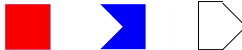
Figure 4.1: Three examples of cuts. The red one represents heat, the blue one water inlet, and the white gas outlet. Other examples of cuts are seen in figure 4.2.
