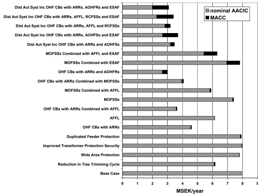
**Figure 1.1:** Sum of maximum annual capital cost (MACC) associated with the implementation of each reliability improvement solution on a test system and the corresponding average annual supply-interruption cost to the test system customers (AACIC).
