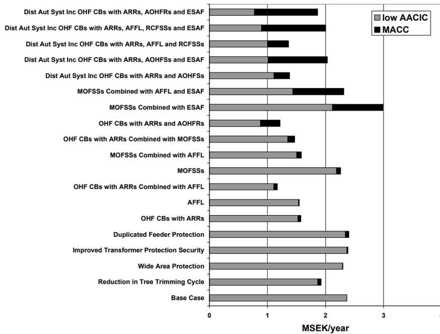
**Figure 10.2:** For each reliability improvement solution applied to the test system, the sum of low average annual interruption cost to the test system customers (AACIC) and maximum annual capital cost (MACC) compared to the low average annual interruption costs to the test system customers when no reliability improvement solution has been applied to the test system (Base Case).
