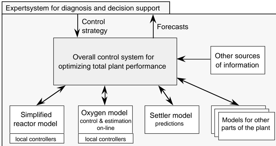
**Figure 4.1** Hierarchical control structure of the WWT process.
