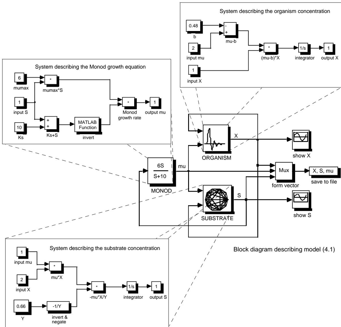
**Figure F.2** Simulink block diagram of the simple model (4.1).
