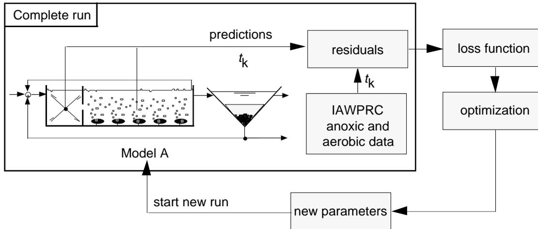
**Figure 5.8** Optimization procedure of the complete 'model A'.
