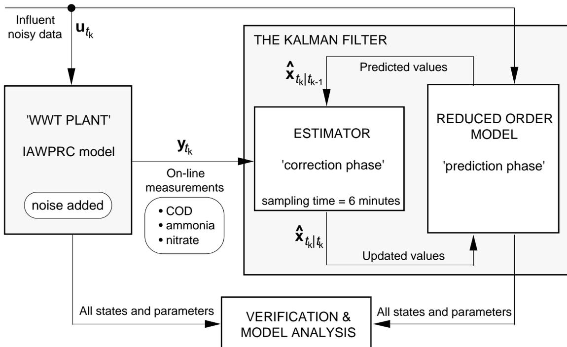
**Figure 4.6** Structured identification using an extended Kalman filter.
