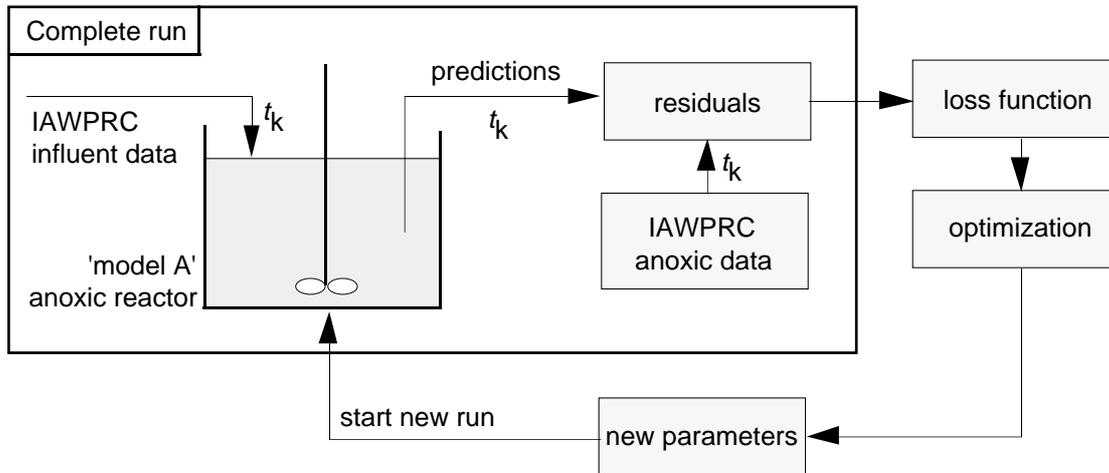
**Figure 5.3** Optimization procedure of an anoxic reactor in unit operation.
