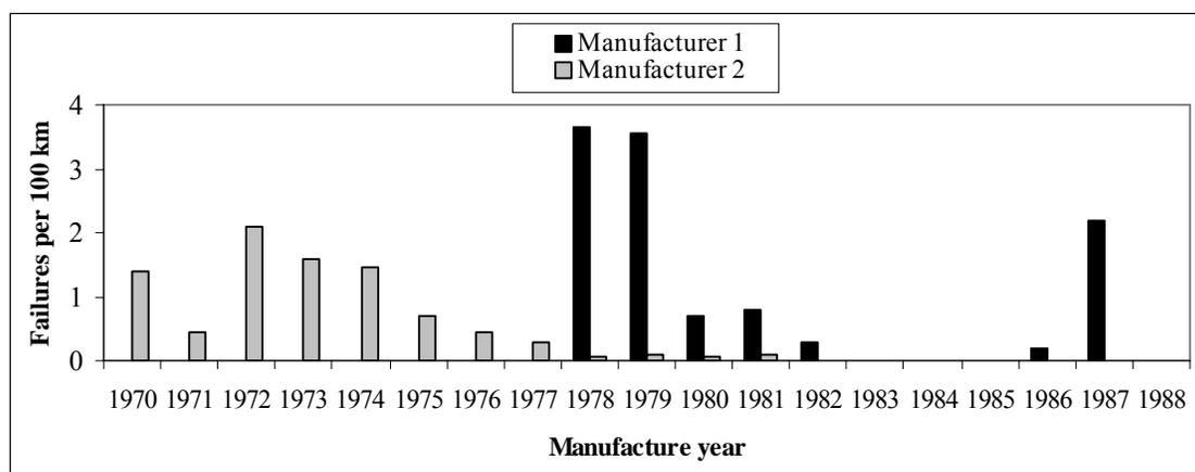
**Figure 5, Manufacture year dependence: XLPE failure rate per 100 km cable, two different manufacturers, Manufacturer 1 data 1978-1988, Manufacturer 2 data 1970-1981**
