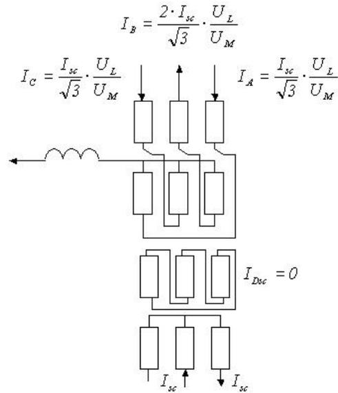
**Figure 5, Two phase short circuit on LV side**
